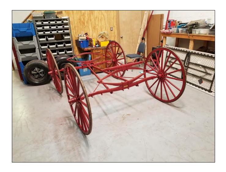
The completed chassis, painted with "Rustoleum Colonial Red", and ready for the box and the front shafts to be mounted.
