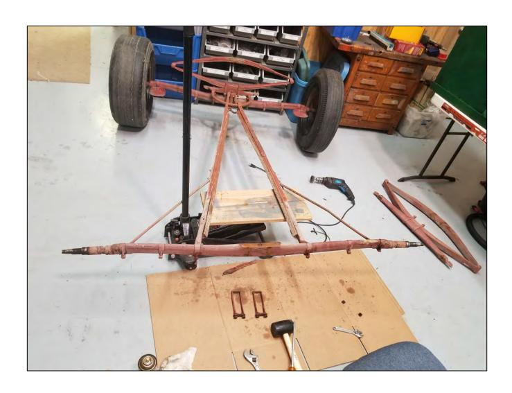
The chassis currently being disassembled.
