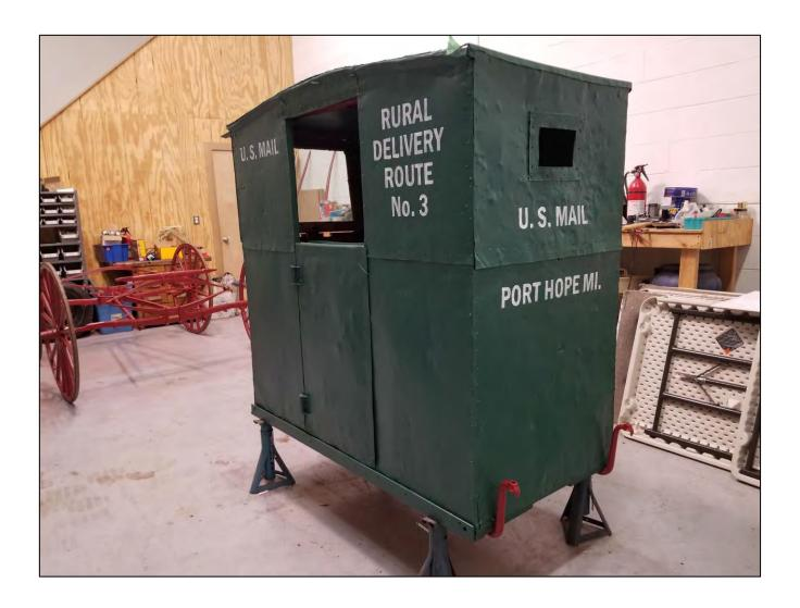
The buggy box now refurbished and ready to be mounted on the chassis. The various bumps, dents and holes were kept intact to preserve the buggy's originality. (the original door handles, "bent nails", were kept as is) The original sliding windows were rebuilt, and the interior painted a combination of green and red.
